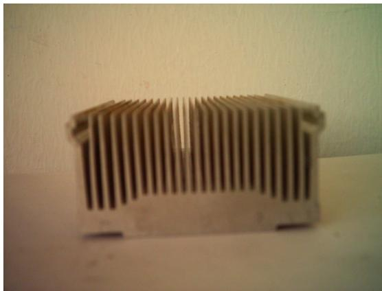
Fig. 2: Conventional heat sink
