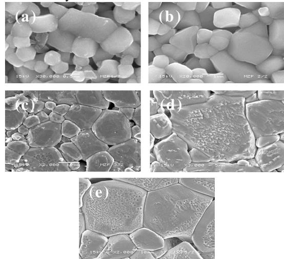
Fig. 3: SEM micrographs of free surfaces of MZF ceramics sintered at (a) 1100 °C, (b) 1200 °C (c) 1300 °C, (d) 1400 °C, and (e) 1500 °C for 2 h with heating/cooling rates of 5 °C/min.
