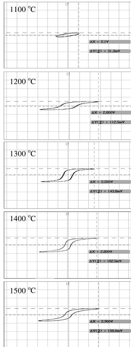
Fig. 5: M-H curves of MZF ceramics sintered at various temperature
