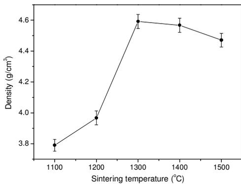
Fig. 2: Dependence of density in MZF ceramics sintered at various sintering temperatures.
