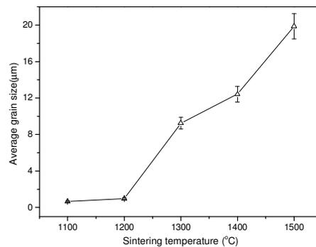
Fig. 4: Average grain sizes of MZF ceramics sintered at various temperature
