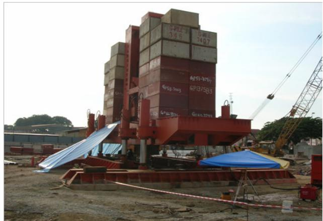
Fig. 6: Static axial compression load test set-up for TP1 at Melaka site, Malaysia
