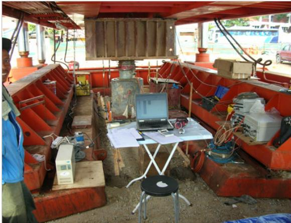
Fig. 7: Instrumentation and monitoring test set-up for TP1 at Melaka site, Malaysia
