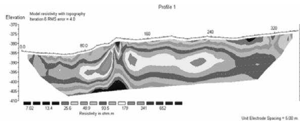
Fig. 5: The resistivity cross-section along profile 1
