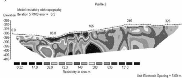
Fig. 6: The resistivity cross-section along profile 2
