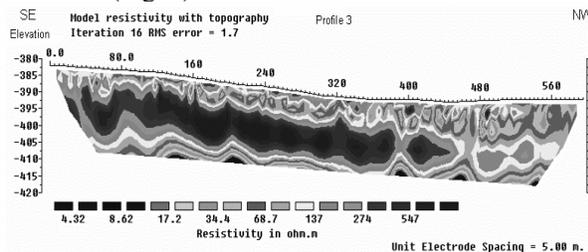
Fig. 7: The resistivity cross-section along profile 3
