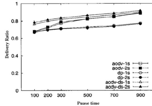
Fig.2 Delivery ratio, 30 sources
