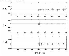
Fig. 4: The DWT Analysis of the three phases of an inrush current at voltage closing angle 36 degree
