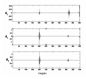
Fig. 6: The DWT analysis of the three phase currents for double phase to ground fault (BC-G)
