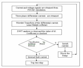
Fig. 2: Flowchart of the proposed Algorithm.
