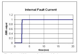
Fig. 8(a): ANN output for internal fault current
