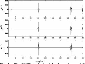
Fig. 5: The DWT Analysis of the three phases of C-G fault current.
