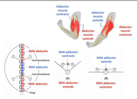
Fig. 5. Biomechanically inspired SMA driven machine
