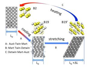
Fig. 2. Thermal and mechanical induced transition in Shape Memory Alloys
