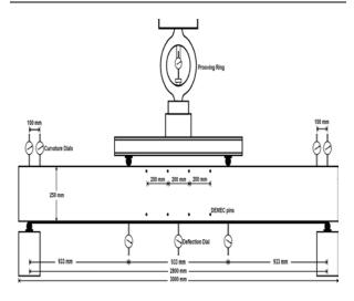
Fig. 1: Loading and Instrumentation Setup
