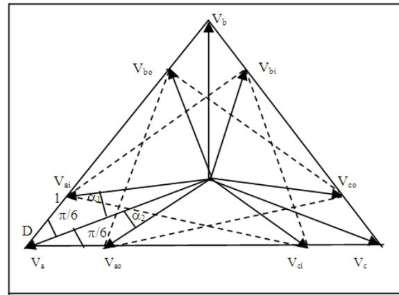
Fig. 4: No-load phasor diagram
