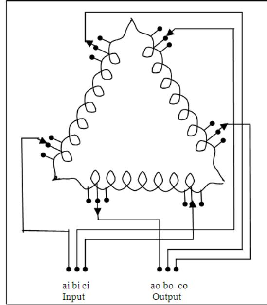
Fig. 3: Delta connected tapped autotransformer
