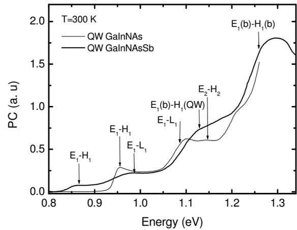
Fig. 1: Room temperature photocurrent spectra of GaInNAs and GaInNAsSb quantum wells
