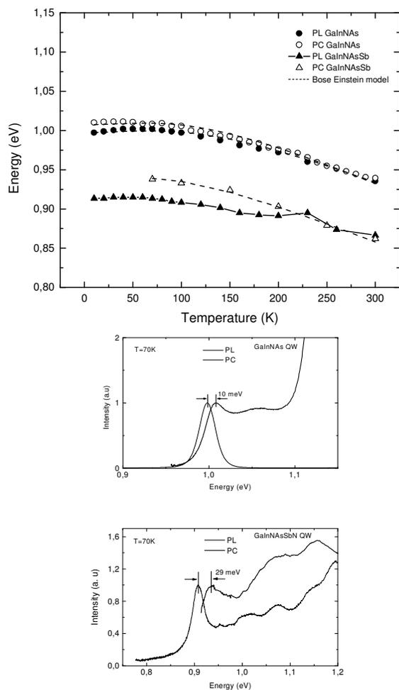
Fig. 5: PL temperature dependence of the emission peak of the GaInNAs (closed circles) and of the GaInNAsSb (closed triangles) QWs. Solid line is a guide to the eyes. Open circles and open triangles represent the  $E_1-H_1$  energies of the GaInNAs and GaInNAsSb QWs respectively. The dashed line is a Bose Einstein fit to the PL and PC measurements of the two QWs. The PC and PL Spectra of the two QWs at 70K are shown in the inset
