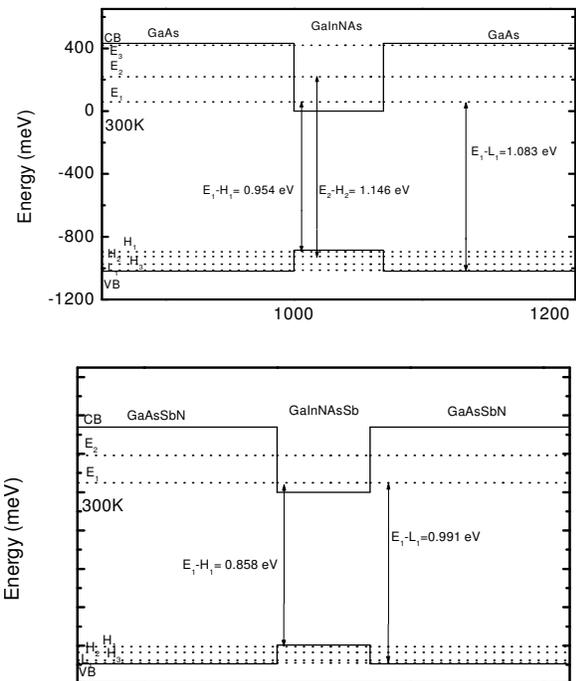
Fig. 3: Room temperature band-edge profiles for GaInNAs and GaInNAsSb quantum wells
