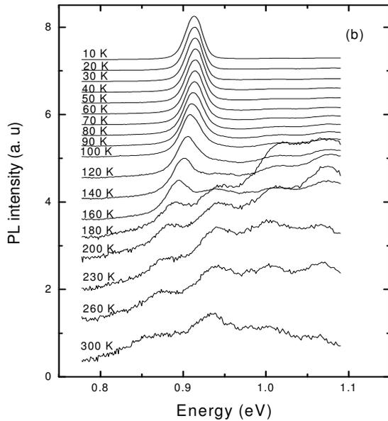
Fig. 4: (a) PL spectra of GaInNAs and (b) GaInNAsSb quantum wells at various temperatures
