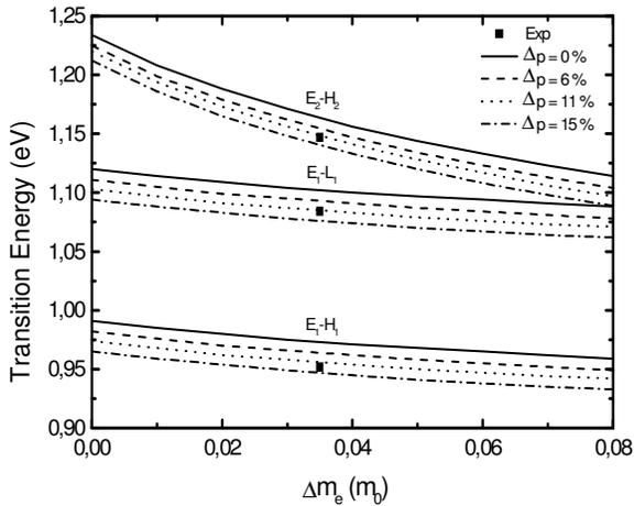
Fig. 2: Room temperature transition energies of GaInNAs as function of the electron effective mass term correction with the theoretical fit (solid and dashed lines) for different  $\Delta p$  shear deformation potential term correction
