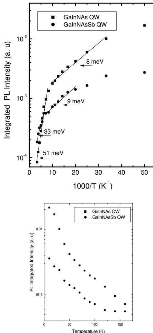
Fig. 6: Integrated PL intensity (log scale) plotted as a function of reciprocal temperature for GaInNAs (closed square) and GaInNAsSb (closed circle) quantum wells
