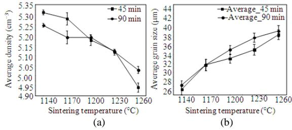
Fig. 2: (a): Average density at different sintering temperature; (b): Average grain size at different sintering temperature
