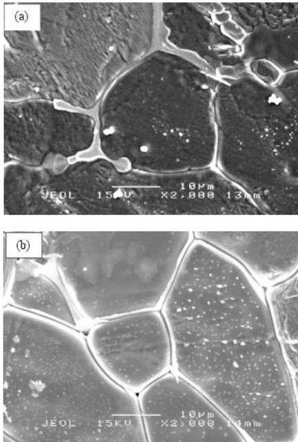
Fig. 3: SEM micrographs of sintered varistor ceramics (a): 1140°C at 45 min sintering time; (b): 1140°C at 90 min sintering time
