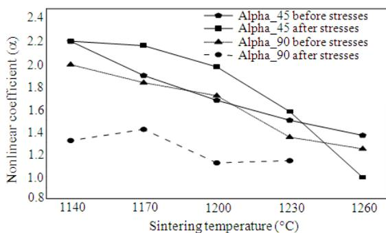
Fig. 6: The variation of average nonlinear coefficient (α) against sintering temperature for 45 and 90 min before and after DC and temperature stresses
