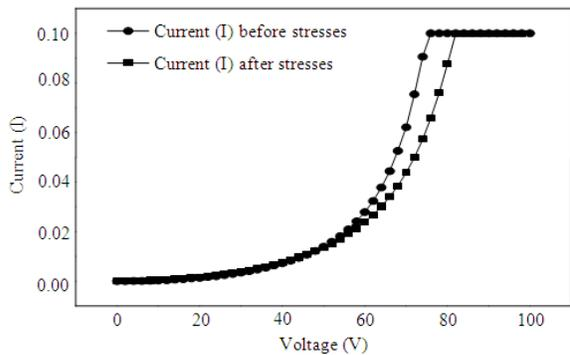
Fig. 5: I-V characteristics of the low-voltage ZnO varistor before and after DC and temperature stresses
