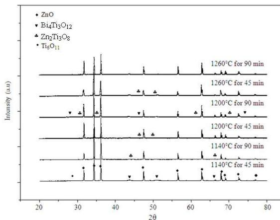
Fig. 1: XRD patterns of varistor ceramics at various sintering temperatures
