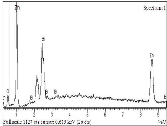
Fig. 4: EDAX micrograph of varistor ceramics at grain boundary
