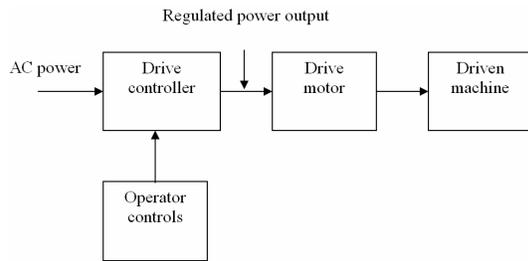
Fig. 6: Functional block diagram
