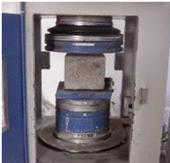
Fig. 11: Compressive strength test
