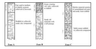
Fig. 2: Lithological log of the surface aquifer
