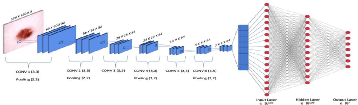
**Fig. 5:** Proposed CNN model architecture
